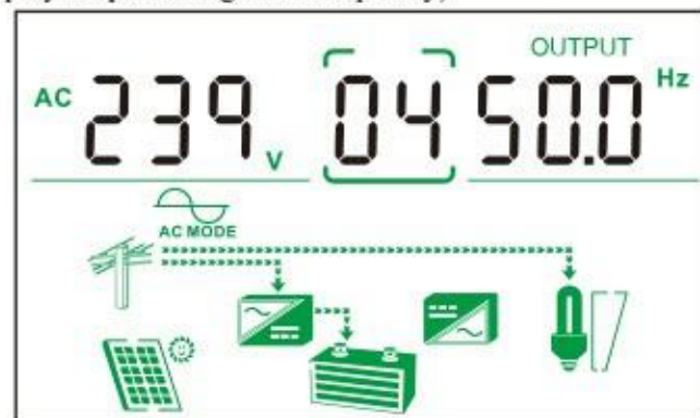
4) Output interface(Display output voltage and frequency)
