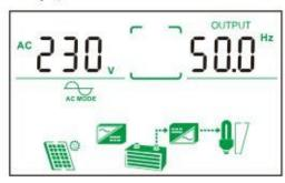
2)Mains working mode (Has PV input, the mains and the PV simultaneously charge the battery)
