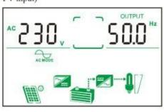
2)Mains working mode (Has PV input, the mains and the PV simultaneously charge the battery)
