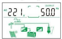
3)Battery working mode (No mains and PV input)
