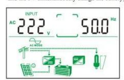
4)Battery working mode (Has PV input but no mains input, only the PV charge the battery)
